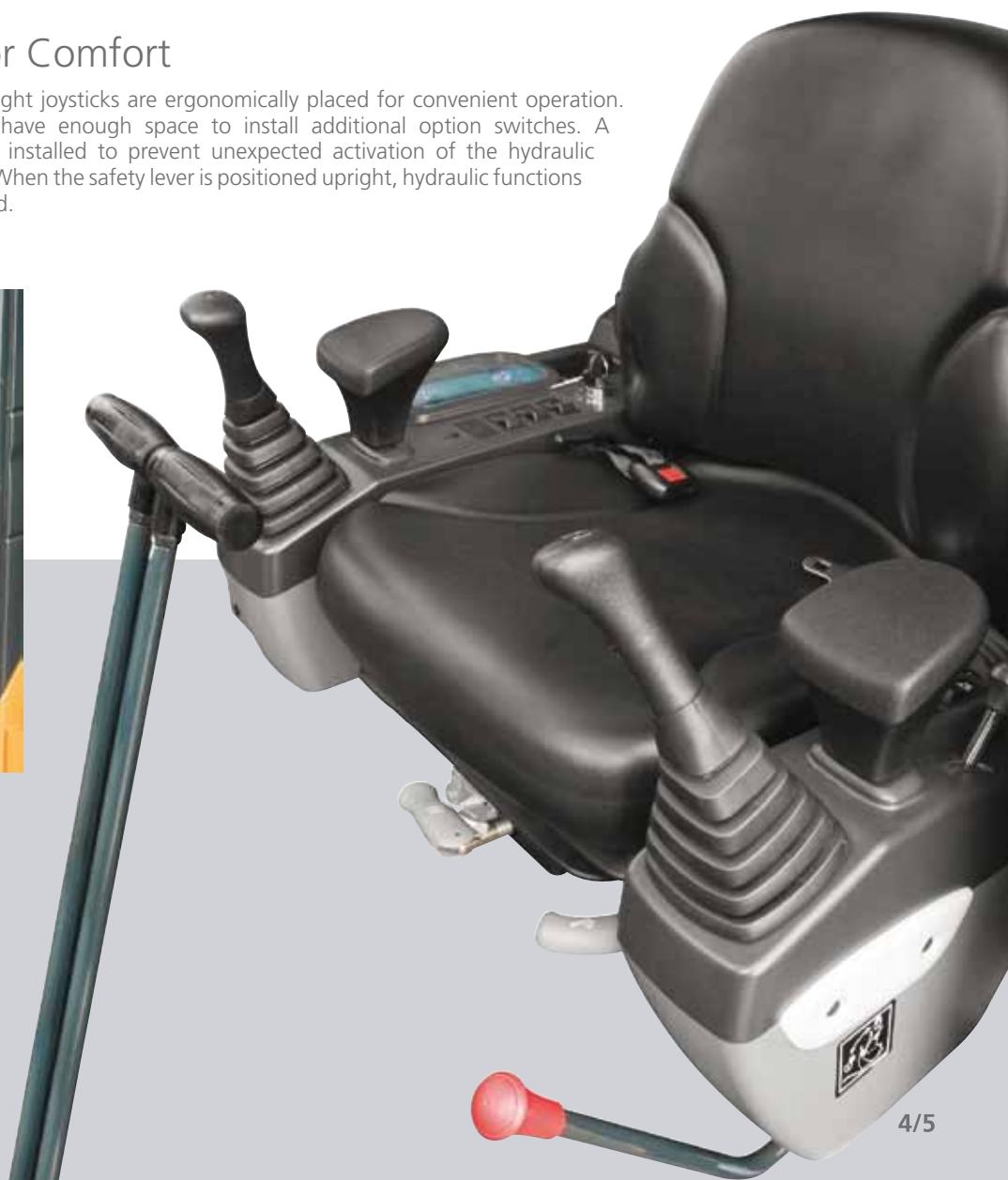
A tiltable left-side console make the operator easier to enter and exit the cab.
