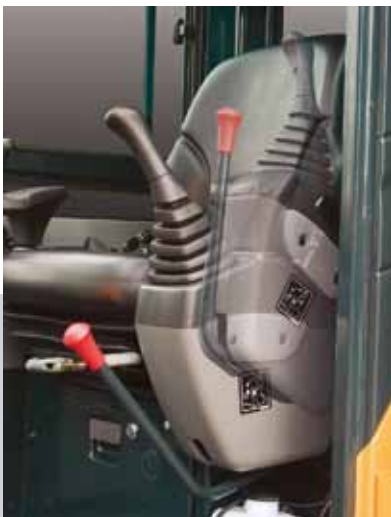
A tiltable left-side console make the operator easier to enter and exit the cab.
