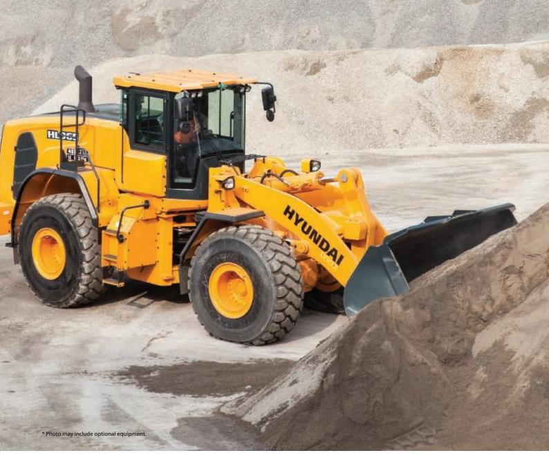
**Net Power** 201 kW (269 hp) / 2,100 rpm **Gross Power** 203 kW (272 hp) / 2,100 rpm Travel Speed 40.0 km/h (24.9 mph) **Operating Weight** 20,100 kg / 44,315 lb
