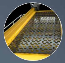
Screen decks Multitude of combinations and configurations for top and bottom decks including e.g. punch plate, befor screen, finger deck, square and elongated meshes – one scalper for different applications.
