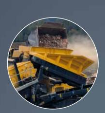
Feed hopper Large feed hopper with a heavy duty multiply belt as standard. The speed of the belt feeder is adjustable to ensure smooth material flow onto the screenbox
