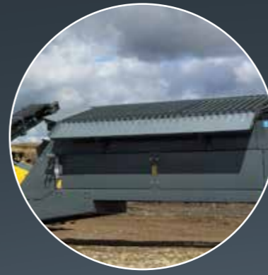
9.2 m 3 hopper, wide loading area Enables the use of wider loading buckets.
