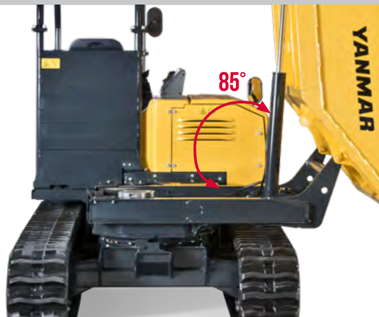
Turning wagon with 180° rotation
