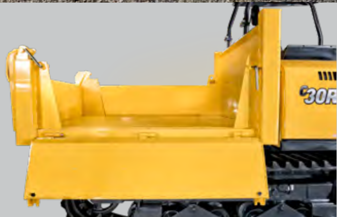
Three-side flaps wagon with rear dumping
